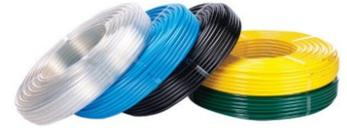
Polyethylene tube is ideal for the transfer of air and liquids. LDPE tube is inert and has excellent resistance to solvents. LDPE is food grade rated to AS 2070.1 (except yellow). **Burst pressure is 3 times working pressure.**
