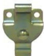
Dummy coupling mounts on the pogo stick or the cab to hold the disconnected suzi coil.
